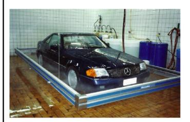
2. Frame stops at hub-cap level. Chemical pumps are activated. Frame rises, spraying water and environmentally safe biodegradable chemical over entire vehicle in 8 seconds.
