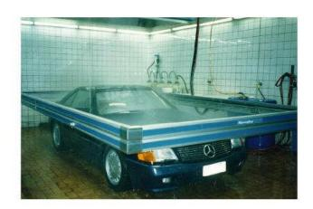
6. Frame completes the final cycle applying protective hi-glo paint sealant to vehicle — producing high shine. Where applicable, optional spot-free rinse sprays deionized water eliminating chamois or towel drying for a "showroom shine".
